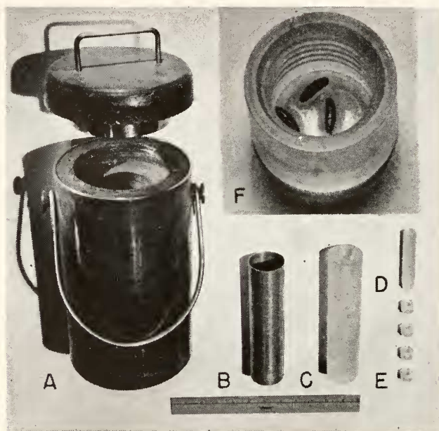
FIGURE 1. Gamma source and accessories. A, lead pig; B, cobalt-aluminum alloy source; C, polystyrene cylinder; D, polystyrene plug; E, polystyrene vessels; F, polystyrene vessel (enlarged) containing grasshopper eggs.
